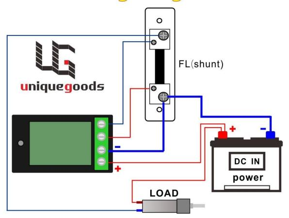
**WARING:** Do not directly connected the power "-" to meter, please power"-" connected to the shunt first, then the shunt wire to meter.
